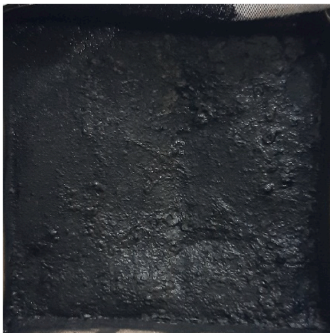
Fig. 1. The picture of the sludge formed on the steel screen.
